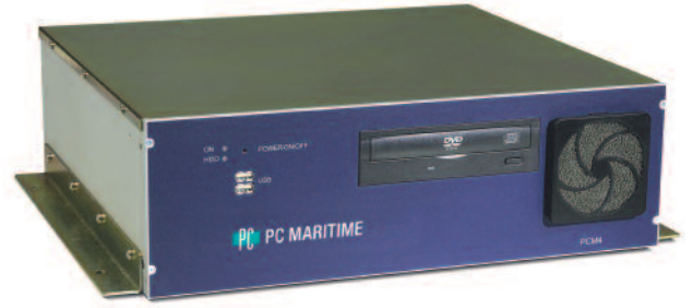
Intel Pentium 4, 2.8GHz, 512Mb RAM, 40 Gb vibration-proof hard drive. Certified to IEC60945 and IACS E10. Brackets are available for horizontal, vertical and 19" rack mounting. Measures 420 x 132 x 380mm.
