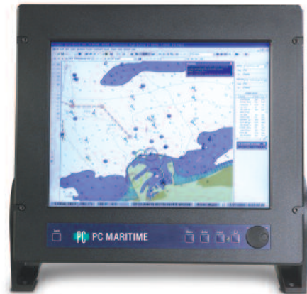
20.1" TFT monitor (larger displays also available) with excellent brightness and contrast levels and direct dimming control. Certified to IEC60945, IEC61174 and IACS E10. Can be panel-mounted or supplied with protective aluminium casing and brackets for desktop, deck-head or wall mounting. Measures 534 x 481 x 223.5mm.
